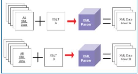
FIGURE 4 An XSLT can be used as an intelligent query to pull specific data from a database.
