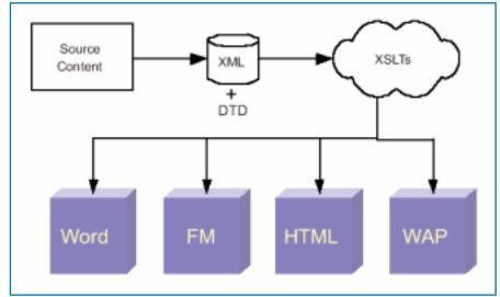
FIGURE 1 Source content is transformed into document instances or learning delivery instances through the XML object components. (FM = FrameMaker document, WAP = Wireless Application Protocol document).
