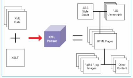
FIGURE 2 XML data and an XSLT are parsed to become a Web site.
