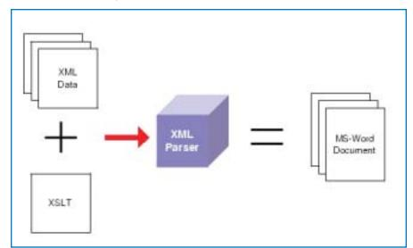
**FIGURE 3** The XML data from Figure 2 and a different XSLT can be parsed to become a Microsoft Word document.
